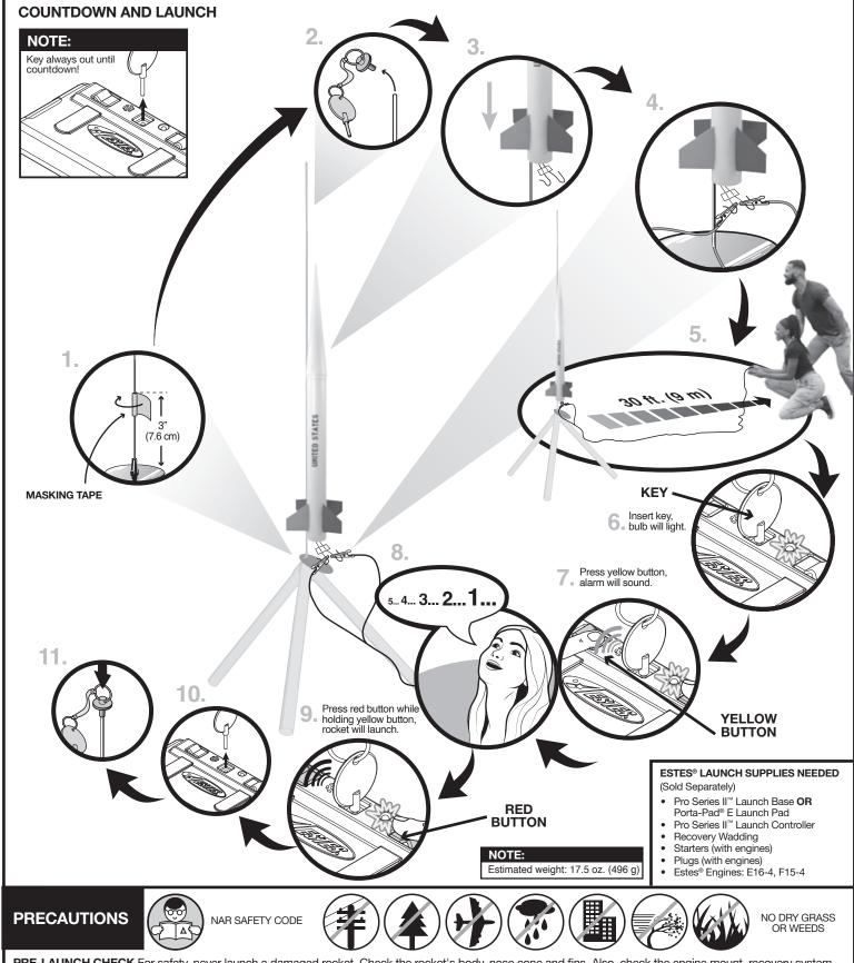
**PRE-LAUNCH CHECK** For safety, never launch a damaged rocket. Check the rocket's body, nose cone and fins. Also, check the engine mount, recovery system and launch lug(s). Repair any damage before launching the rocket.
